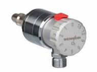
Flow dosage setting knob for central gas system in ermergency vehicles, clicks into place at settings for 1, 2, 3, 4, 5, 6, 9, 12, 15 L/min, incl. one (1) connection nozzle with swivel nut, straight, Ø 6 mm, UNF 9/16" (WM 31122)
