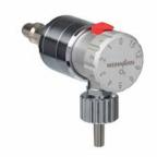
Flow dosage setting knob for central gas facility in emergency vehicles, clicks into place at settings for 1, 2, 3, 4, 5, 6, 9, 12, 15 L/min, incl. one (1) connection nozzle with swivel nut, straight, Ø 6 mm, UNF 9/16" (WM 31122)
